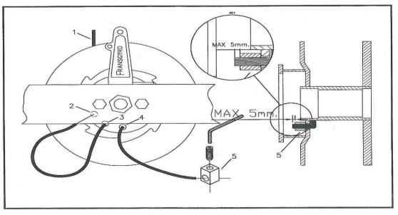
Drawing "B" Attaching cable to wire drum
