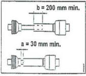
The P.T.O must be cut to a proper length, so it does not "bottom out" and bind. Remove the PTO to perform this operation. If the PTO is not cut to the proper length, it may cause damage to the PTO, gearboxes etc. See illustration for proper measurements. a = clearance when attached to tractor; should be 30mm /1.20 inches b = overlap; should be 200mm / 7.87 inches
